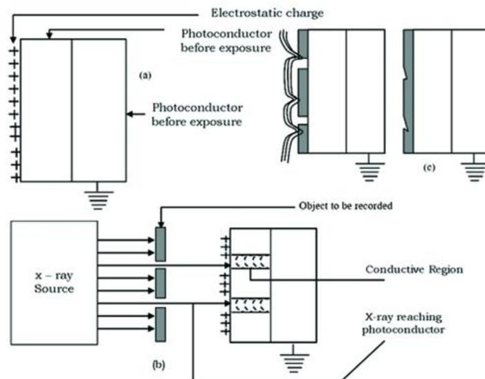
A schematic figure of the Xeroradiography process by Rawls and Owen<sup>19</sup>: (a) The charged photoconductor acting as an insulator; (b) Exposure ensures charge to be conducted away from the surface; (c) particles collect in charged areas, giving positive image<sup>[4]</sup>
