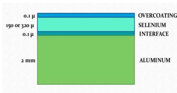
A schematic figure of a xeroradiography plate
