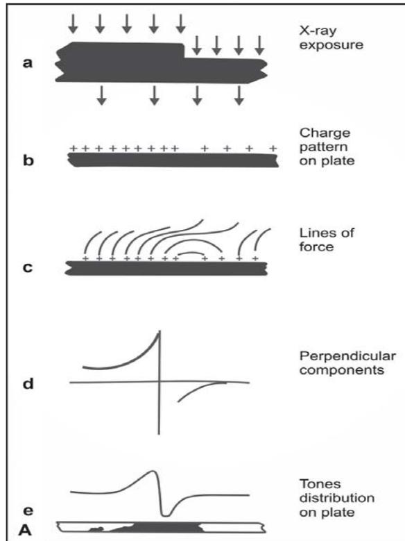
An X-ray beam passing through an object is differentially attenuated according to the absorption characteristics of the object. **B.** The disruption of transmitted X-ray photons alters the charge pattern on the Xerox plate. **C.** Lines of the force produced as a result of the difference in charge densities on the plate surface. **D.** These lines of forces have perpendicular components. **E.** These components affect the distribution of the toner particles on the plate
