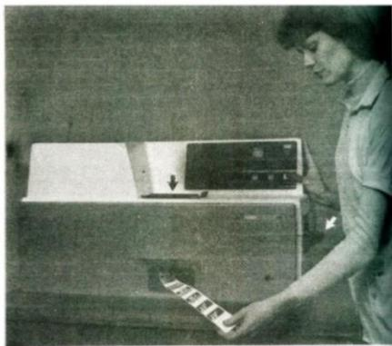
FIG. 13-26. Dental 110 system showing output station (black arrow) and input station (white arrow).
