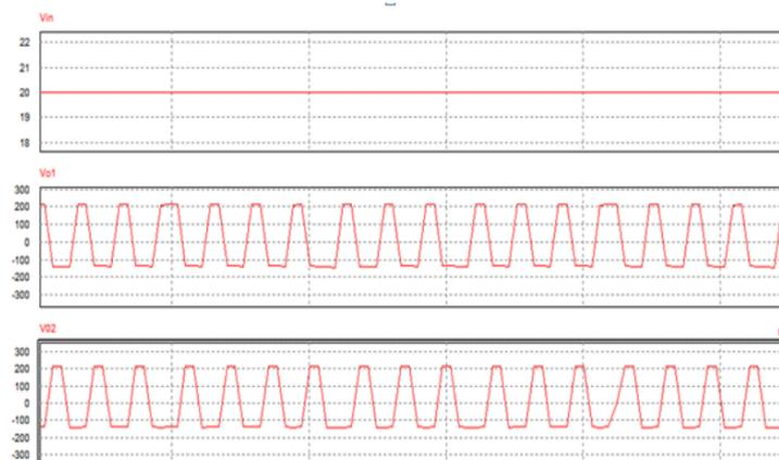
**Fig 3. Input Voltage ( $V_{in}$ ) and Voltage across flyback converter 1 and converter 2.**
