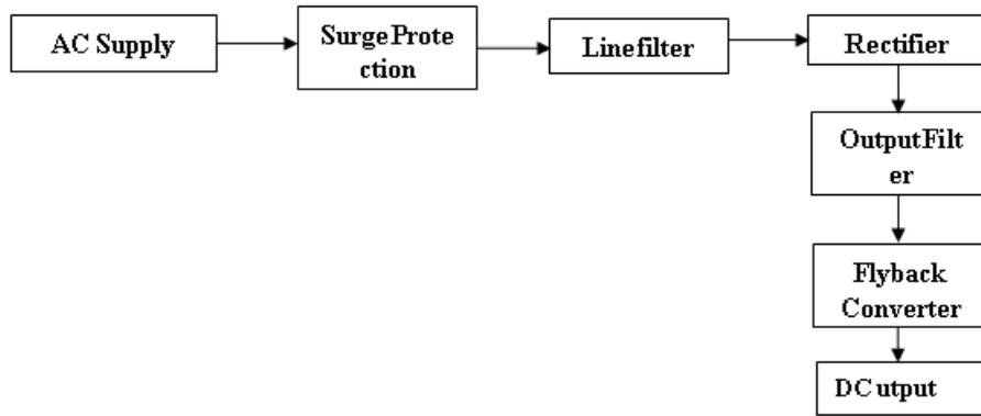
**Fig.1 Conventional Flyback PFC Converter**
