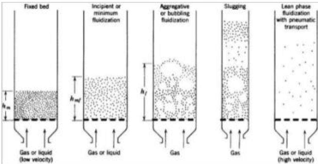
Fig.1.Mechanism of Fluidized Bed Reactor
