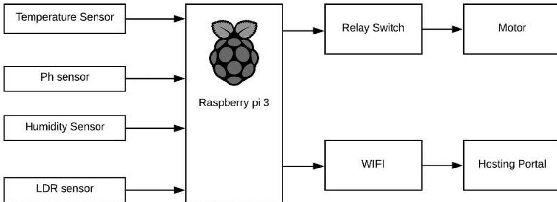
Figure 6 Block Diagram of the System
