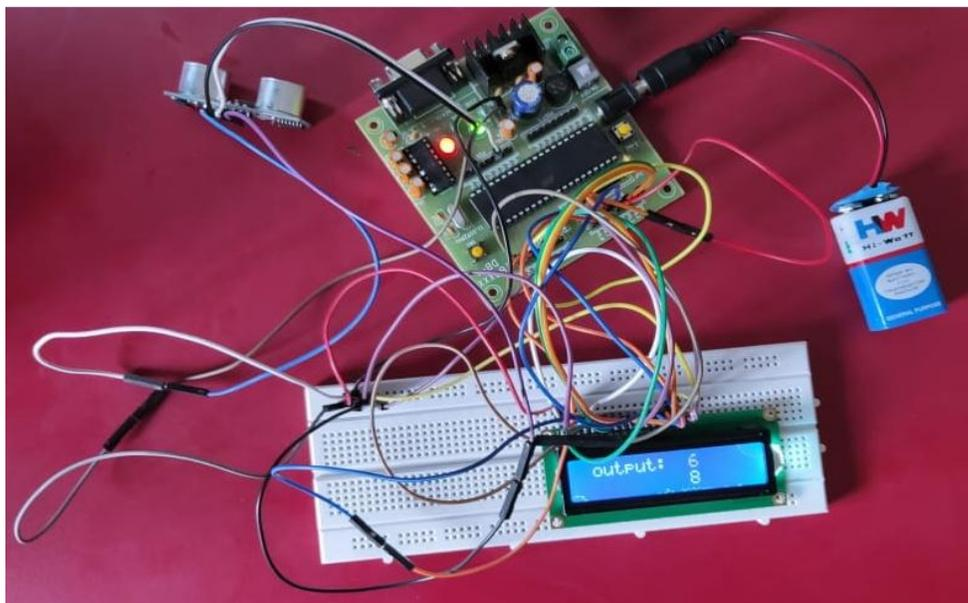
Figure6. Ultrasonic sensor interfacing with 89c51
