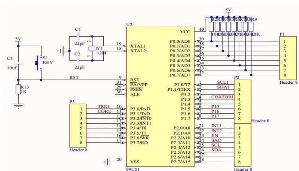
Figure3. Circuit schematics of AT89c51
