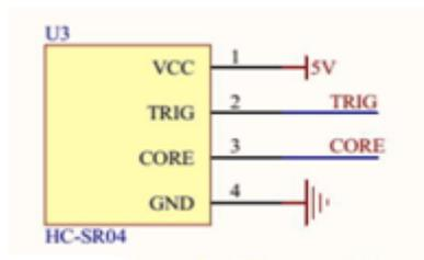
Figure2. Circuit schematics of HC-SR04 ultrasonic distance sensor
