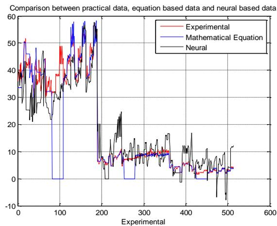
Figure 5 Comparisons between experimental data, ANN and RSM for predicted strength
