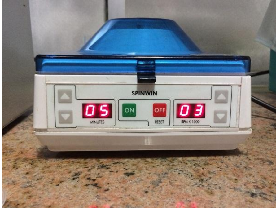
Figure-1 Samples collected are centrifuged at 3000 rpm for 5 minutes
