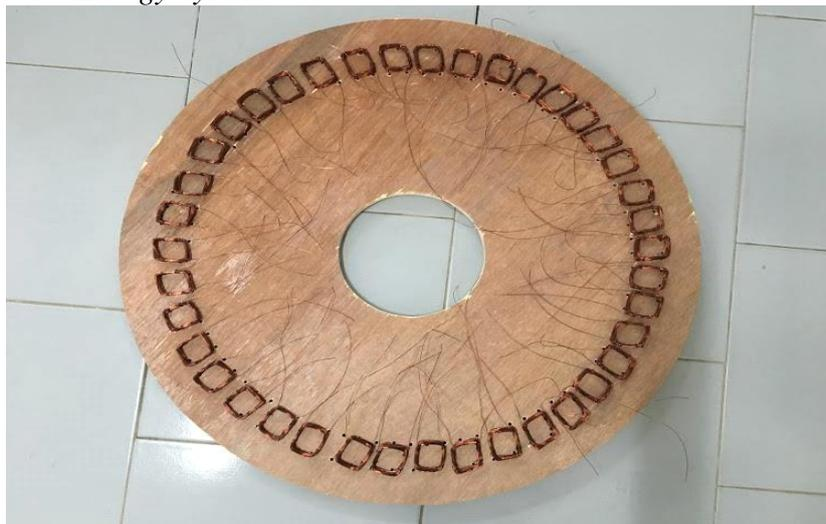
Fig.4 Coils Wound on a Wooden board acts as Stator
