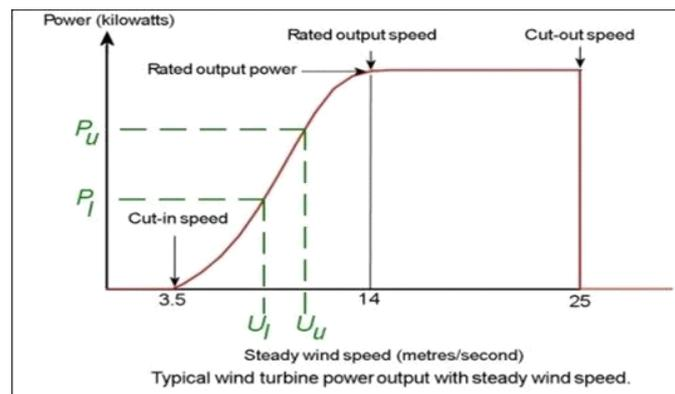
Graph.3 Variation of power with the with respect to the wind speed
