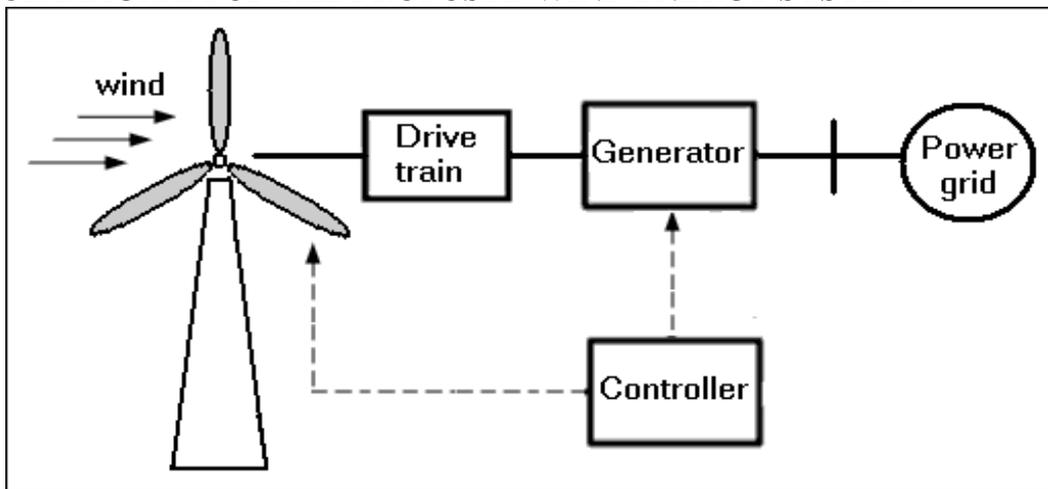
Fig 9. General block diagram of wind power generation
