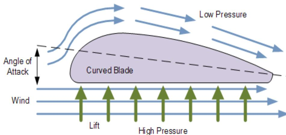
Fig.8 Curved Blade Air Flow and Performance
