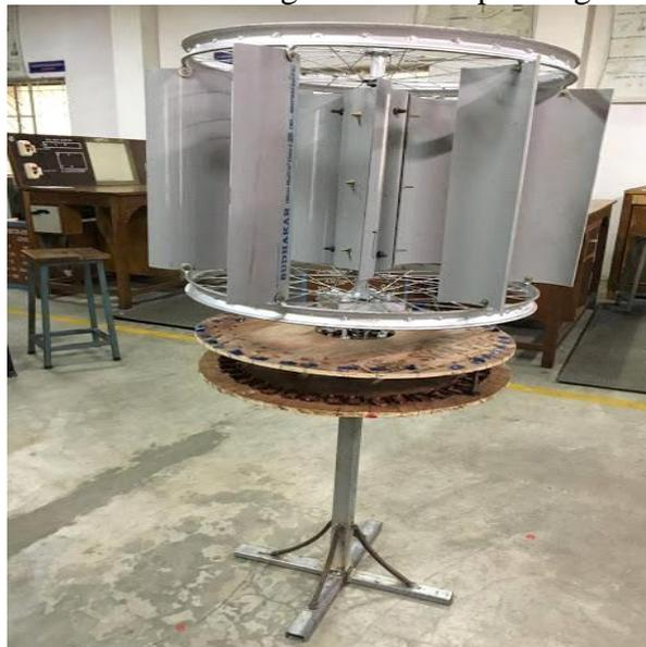
In this, the two stator boards are coupled by nuts and bolts with the rotor placed between them. Fig.10 wind turbine based power generator
