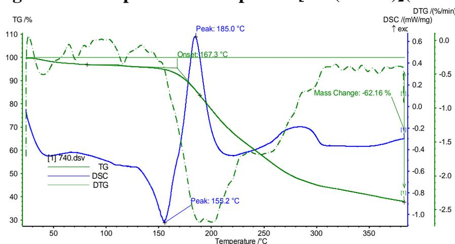
**Figure 4. Thermograms of compounds [Cu (PNBA)<sub>2</sub>(MEA)<sub>2</sub>]**
