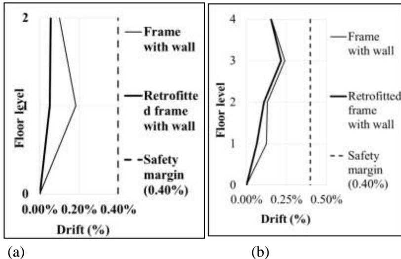
Figure 7. (a) Maximum inter-story drift of Engineering Building 2 at longitudinal direction for 2013 Bohol response spectrum (b) Maximum inter story drift of Administration Building at longitudinal direction for 2013 Bohol response spectrum.
