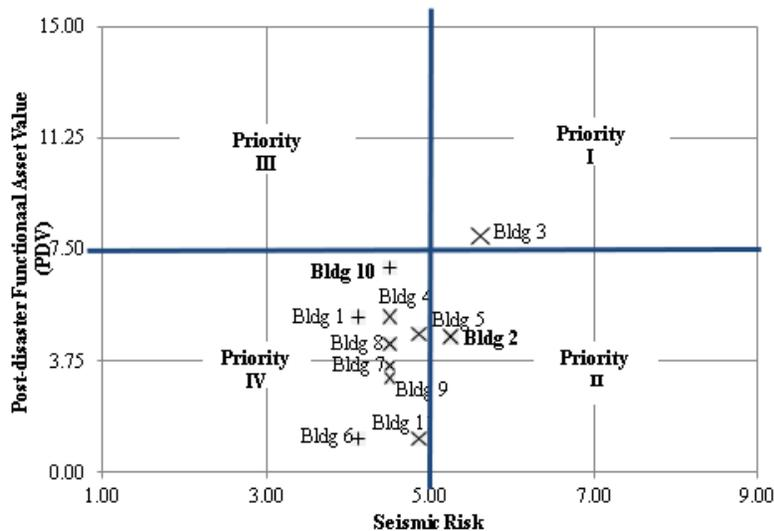
Figure 1. Seismic risk scores are plotted against the PDV values in x and y axis, respectively.
