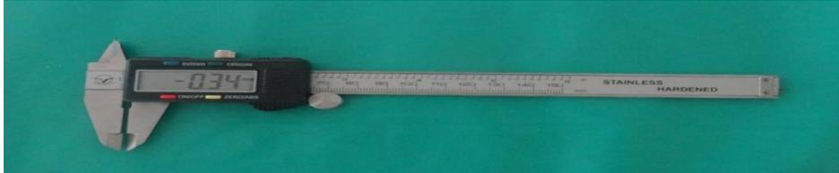
Figure 1: Digital vernier caliper
