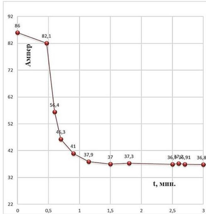
**Fig. 1. Dependence of the current strength on the mixing time for a concrete mixture with OK = 3.0 cm (planetary concrete mixer 2250 / 15001).**
