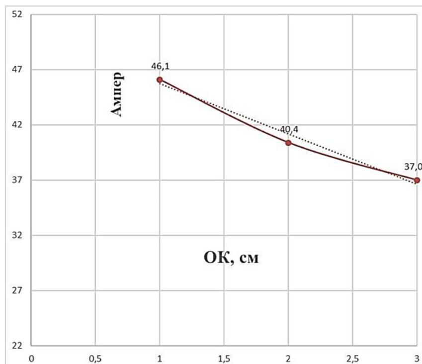
**Fig. 3. The relationship between the values of the current strength (A) at the optimal time for mixing concrete mixtures (from Fig. 2)**
