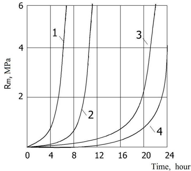
Fig. 1. 1- PC M400, 2- C + 0.1% water repellent on fly ash, 3- C + 0.1% on Gliezh, 4- C + 0.1% on quartz sand.
