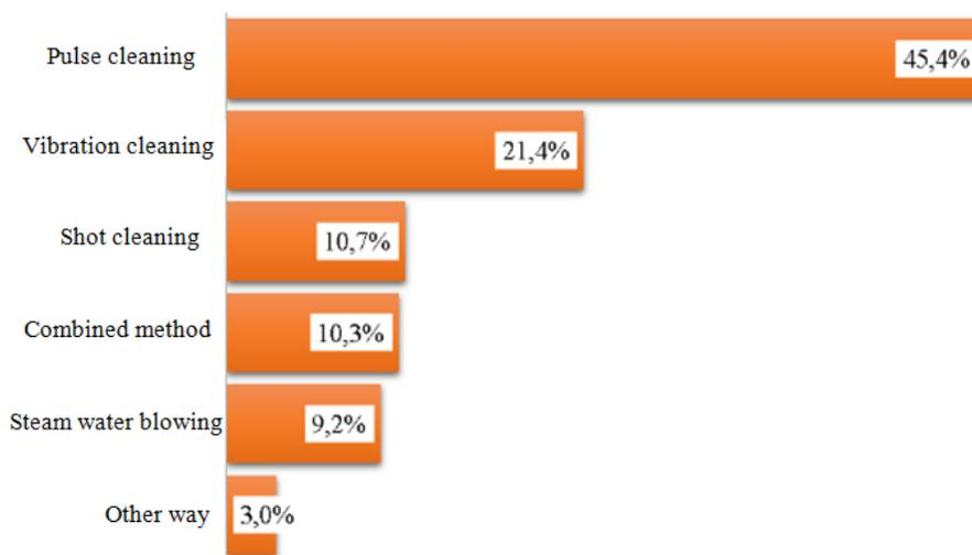
Picture 1: Fraction of applications of individual methods for cleaning the heating surfaces of exhaust heat boilers
