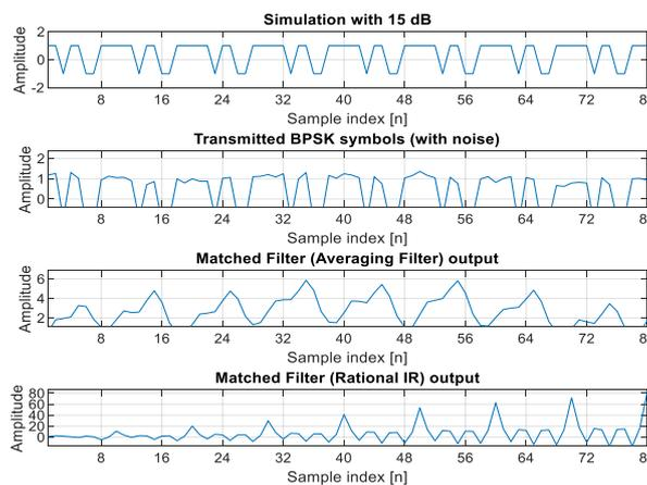
Fig-5: Simulation waveform for BPSK data transmission
