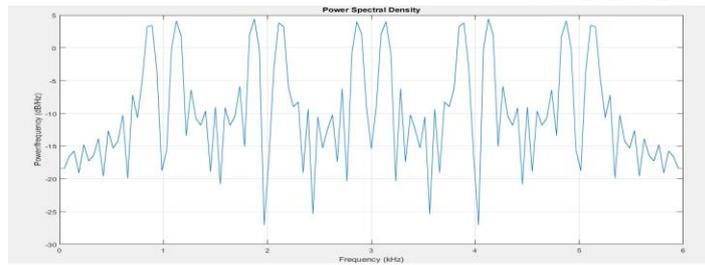
Fig-4: Used and unused spectrum for cognitive channels
