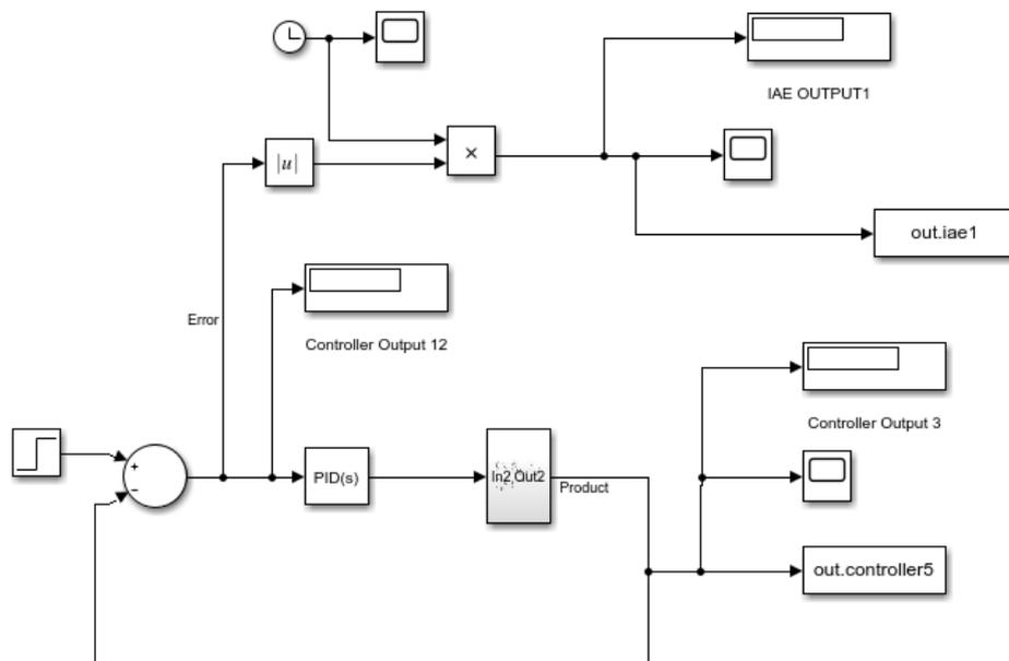
Fig 7.IMC based PID Controller
