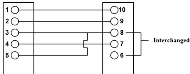
Fig 3. Interchange Circuit
