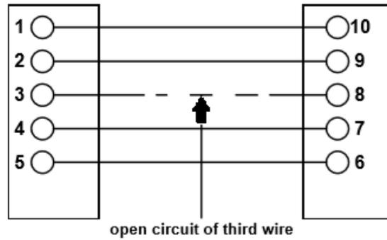
Fig 2. Open Circuit
