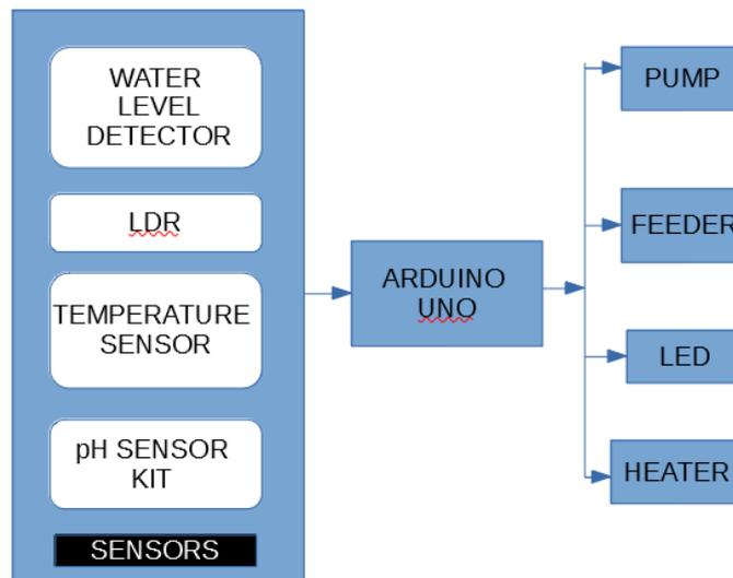
The model hardware is developed on an Arduino uno board consisting of the following sensors
