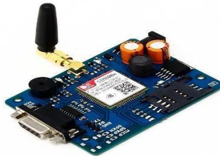
Fig3: GSM Module
