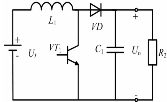
Figure2. Topology of Boost Converter.
