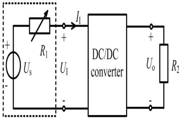
Figure1. The diagram of solar cells simulator
