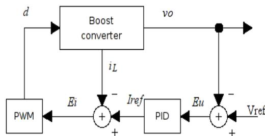
Figure3. Control system configuration
