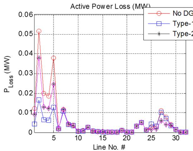
Figure 1: Active power loss comparison for DG (Type-1, Type-2) & without DG placement
