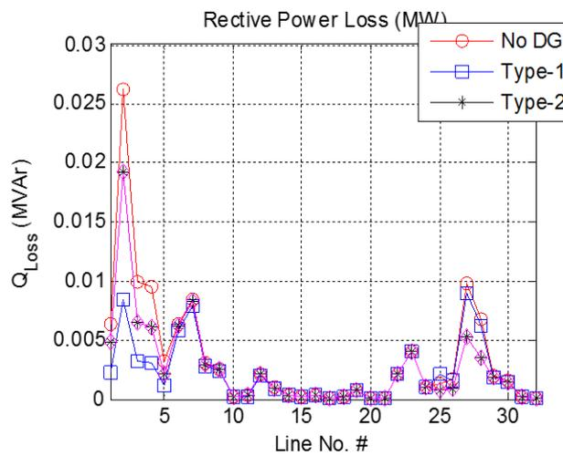
Figure 2: Reactive power loss comparison for DG (Type-1, Type-2) and without DG placement
