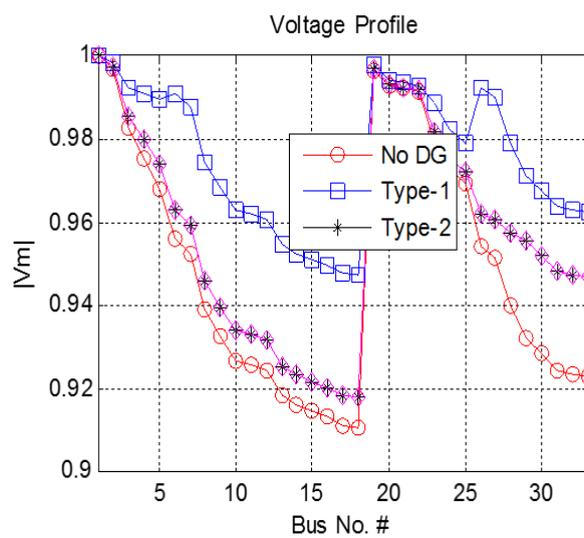
Figure 3: Voltage profile for DG (Type-1, Type-2) and without DG placement
