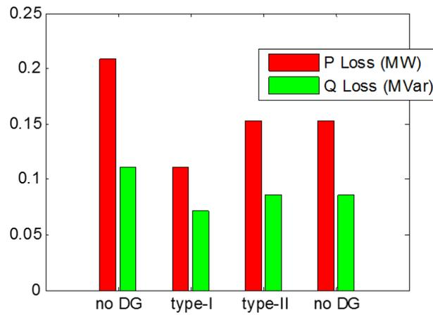
Figure 4: Bar graph for active and reactive power loss minimization with DG (Type-1, Type-2) and without DG placement
