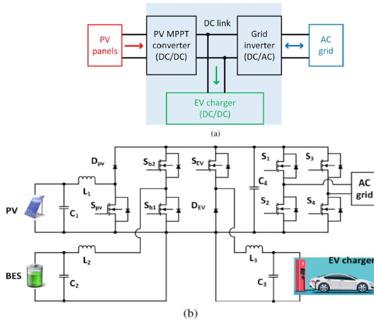
Figure1: Multi terminal converter system construction, (a) EVL is connected to PV array without battery
