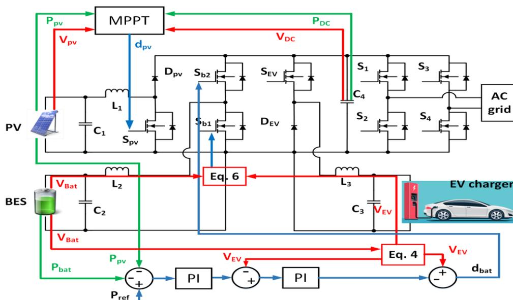
Figure 3. Control diagram of PV and battery is connected to EVL.
