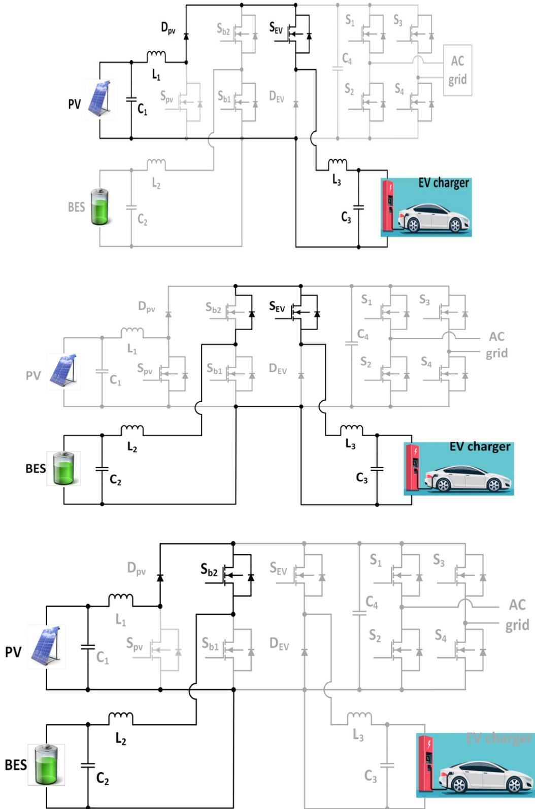
Fig.2: Multi terminal converter system operation modes, (a) PV supply is equal to EVL (b) Battery energy storage supply EVL charging during lack of PV power (c) PV power excess the EVL and charging mode of battery
