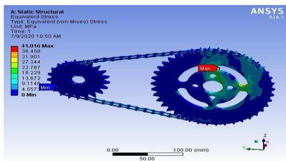
**Material: EN 32 Steel At speed -40 km/hr**
