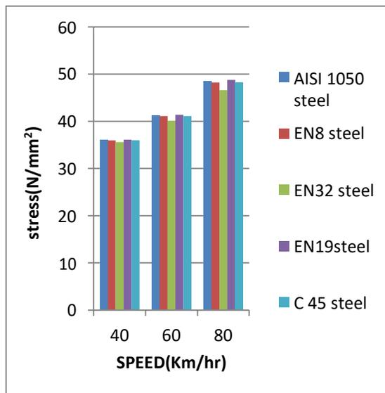
Plot 2: shows comparison of materials and speed versus stress
