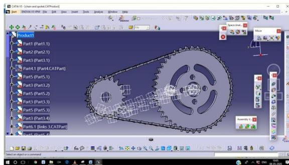
Fig: 3D model of chain sprocket
