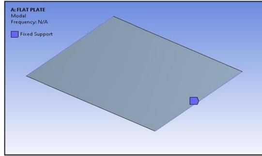
Figure.3. Applying Boundary condition on 2 mm plate
