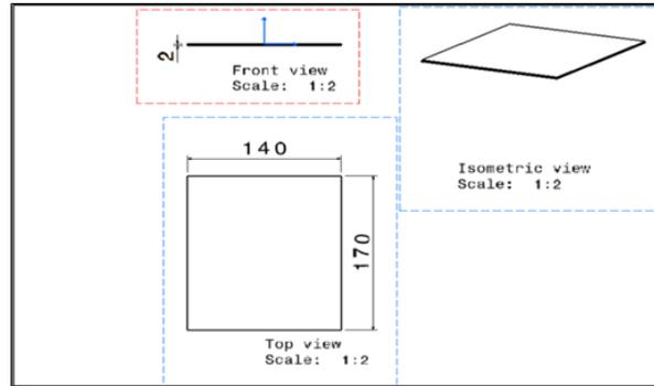
Figure.2. drafting of 2 mm plate
