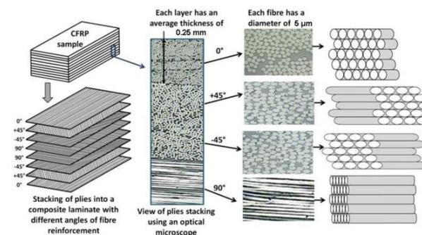
Figure 1.1: Lay-up process of CFRP and properties of CFRP.
