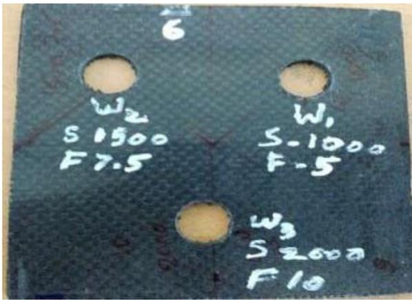
Fig.7. 6 layers, thickness 2.0
