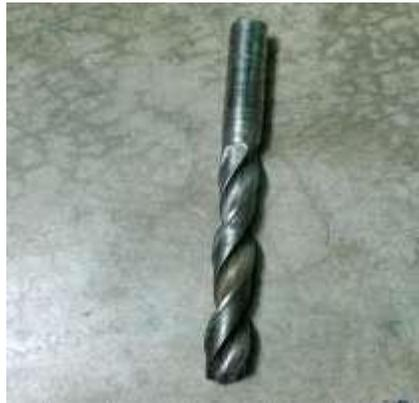
Figure.4. High Speed Steel DrillBit(12mm)
