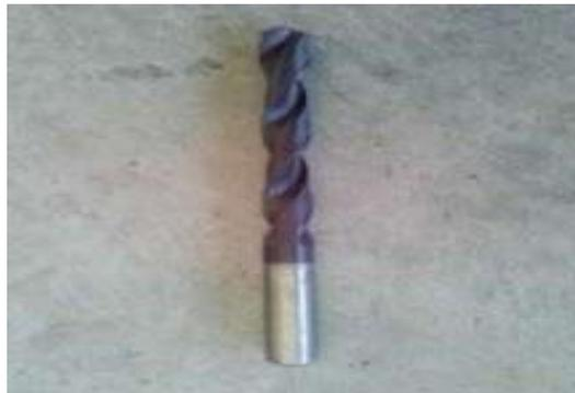
Figure.5. HSS Drill bit with TiAlN (Single coated)
