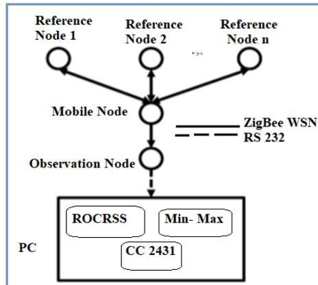
Figure 1: Dataflow in existing location calibration techniques
