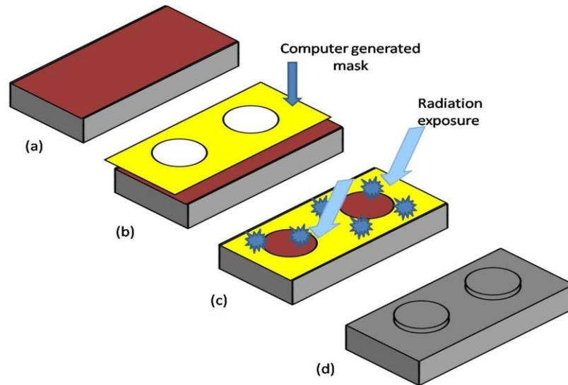
**Figure 4: (a) Coating of a photosensitive resist material on substrate, (b) transferring of a computer generated mask on the resist, (c) Exposure to UV light or a light source, (d) Formation of desired pattern after removal of photosensitive resist**
