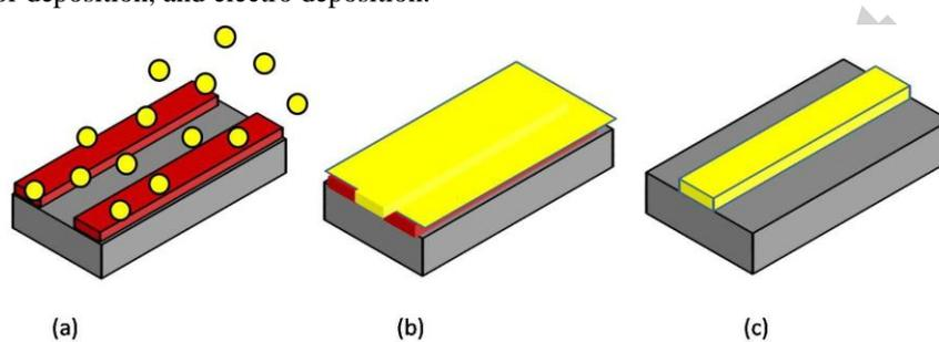
**Figure 3: (a) Deposition of film forming material on substrate, (b) formation of thin film on substrate, (c) Removal of the photoresist material to give desired film**
