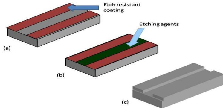
**Figure 5: (a) covering the substrate with etch resistant material, (b) reaction of the etchant with uncovered substrate, (c) Formation of a pattern after removal of etch resistant material.**
