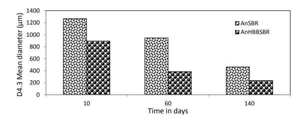
Fig. 4. Anaerobic granule size distribution after 10, 60 and 140 days of AnHBBSBR operation De Brouckere mean particle diameter (D4.3)
