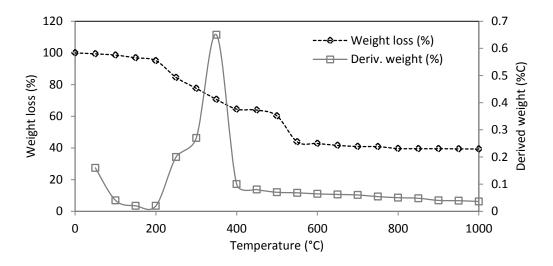
Fig. 5.Thermo gravimetric analysis of paper mill sludge
