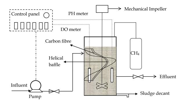
Fig. 1.Schematic setup of bioreactor
