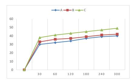
Figure 2: Oil release profile of PEG encapsulated nanoparticles with increase in time
