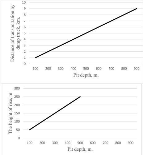
Fig. 1. Relationship of transport distance and lifting height with the depth of the quarry.
