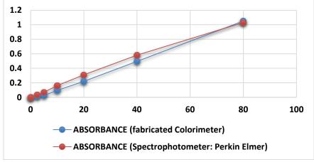
**Chart 4:** Linear curve shows the accuracy of the fabricated calorimeter and P-E Spectrophotometer.
