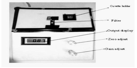
Figure 1(a): the photographic films of as fabricated Colorimeter
