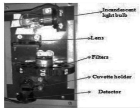
Figure 1(c) Photographic film of as fabricated colorimeter using incandescent light source.
