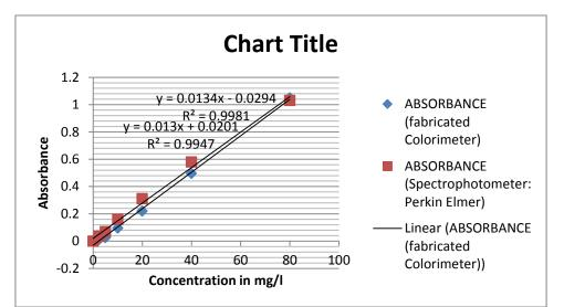
**Chart 1:** Determination of Absorbance with fabricated Colorimeter and Spectrophotometer Perkin Elmer.
