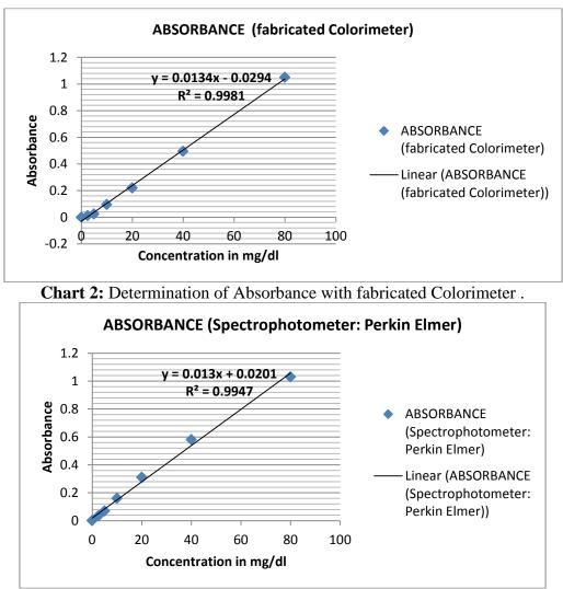
Chart 3: Determination of Absorbance with Spectrophotometer Perkin Elmer.
