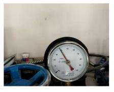
(28 days)Maximum flexural strength achieves with 4% metakaolin and 0.3% vetiver fiber P=38 kilo newton, minimum length of fracture from support(a)=21cm l=60cm b=15cm, d=15cm formula used fck=pl/bd<sup>2</sup>
