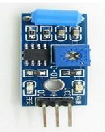
Fig 6: Vibration Sensor
