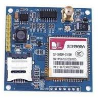
Fig 5: GSM Module
