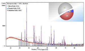
Figure 2. Phase composition of a mesoporous sorbent based on tetraoxysilane and TiO<sub>2</sub>
