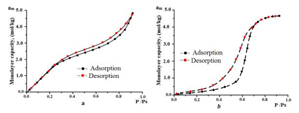
Figure 5. Study of the sorption isotherm of vapors of benzene (a) and water (b) at a temperature of 473 K and a residual pressure of  $1.33 \cdot 10^{-3} \text{ Pa}$ .
