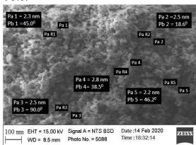
Figure 3. Surface of mesoporous sorbent obtained at 35 °C
