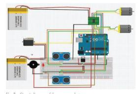
Fig.2. Implementation of prototype using Arduino
