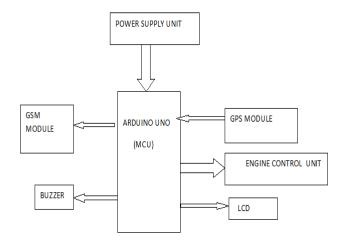
Fig 1.Blok Diagram of fisherman safety system
