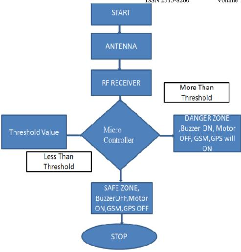
Fig 5: Flowchart of Fishermen border protection system
