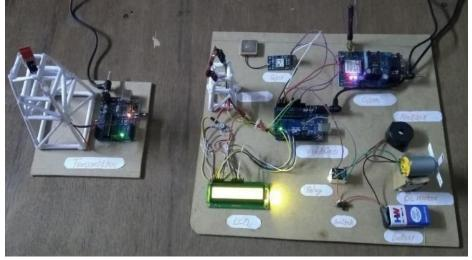
Fig 7: Complete working module of border protection system
