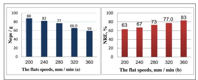
Fig. 1.The effect of the speed of the flats on the removal of Neps / g. and Neps removal efficiency, NRE%.
