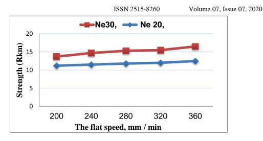
Fig. 6.Effect of flat speed on yarn strength (Rkm) / cN / tex.
