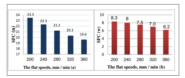
Fig. 2.The effect of flat speed on short fibers by the amount of SFC (n) (a) and short fibers by weight of SFC (w) (b).
