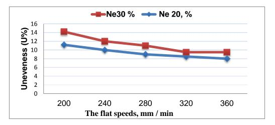
Fig 4.The effect of the speed of the flats on the unevenness of the yarn Ne20 and Ne30. Defects and defects of yarn (IPI). Figure 5 (a) to (d) depict yarn defects. Here we look at thick places, thin places and Neps.
