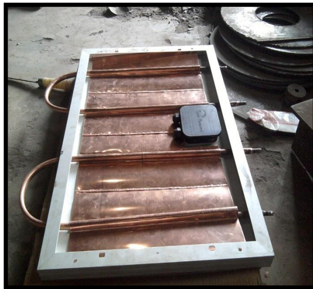
Figure 1. Back View of the PV/T (cooled) System
