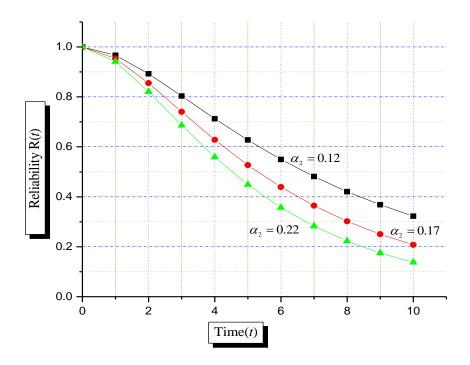
Figure 3 Reliability w.r.t.  $\alpha_2$  vs. Time unit (t)
