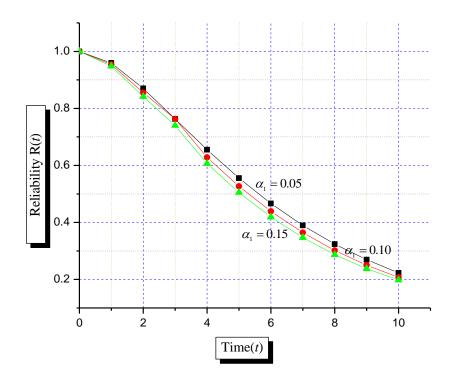
Figure 2 Reliability w.r.t.  $\alpha_1$  vs. Time unit (t)
