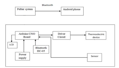
Figure 1. Block Diagram
