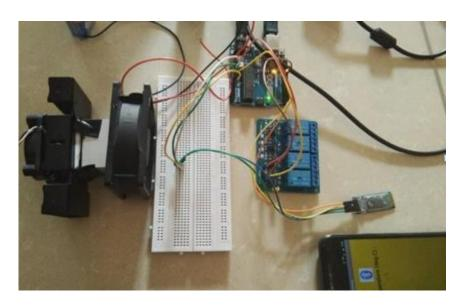
**Figure 3**. LM-35 temperature sensor, HC-05 Bluetooth module connected to display the temperature on the android phone.
