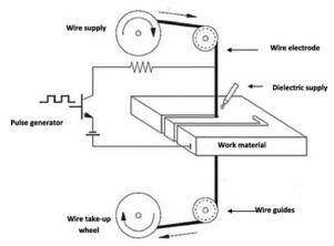
Figure 1 Working Principle Wire cut EDM Process [11]
