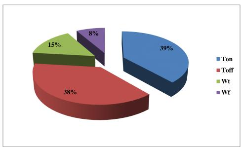
Figure 6: Power of control in percentage of identified parameters on Surface Rough
