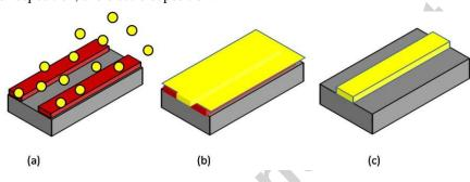
Figure 3: (a) Deposition of film forming material on substrate, (b) formation of thin film on substrate, (c) Removal of the photoresist material to give desired film
