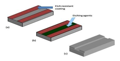
Figure 5: (a) covering the substrate with etch resistant material, (b) reaction of the etchant with uncovered substrate, (c) Formation of a pattern after removal of etch resistant material.
