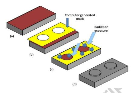
Figure 4: (a) Coating of a photosensitive resist material on substrate, (b) transferring of a computer generated mask on the resist, (c) Exposure to UV light or a light source, (d) Formation of desired pattern after removal of photosensitive resist
