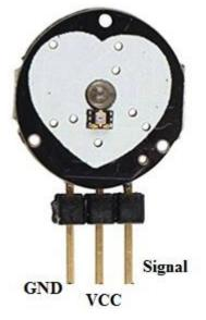
Figure 3: Heart Rate Sensor
