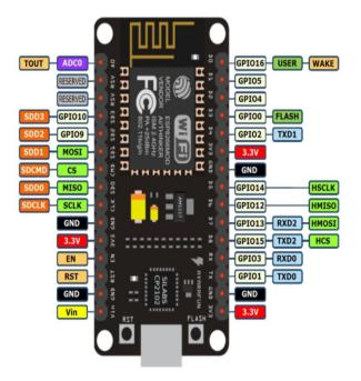
Figure 1: Pin-out of Node MCU
