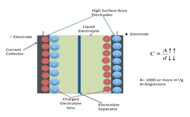
Fig. 1: Schematic Diagram of Supercapacitors
