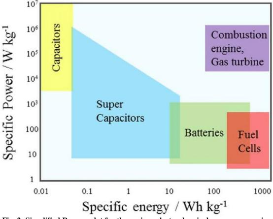
Fig. 2: Simplified Ragone plot for the various electrochemical energy conversion systems.
