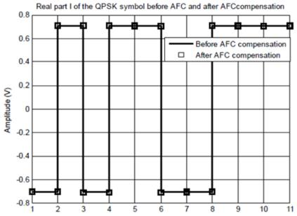
Figure 2 Phase symbol before and after AFC
