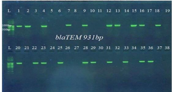
Figure (5): Agarose gel electrophoresis of PCR products for the resistance genes *bla*TEM. Lane L: 100bp DNA ladder; 1-38 *K. pneumoniae* isolate. Positive result in 1,2,4,7,9,12,13,15,16,18,20,22,23,25,28,29,31,33,35 and 36.
