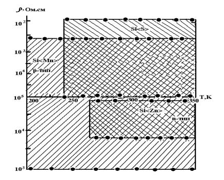
Fig. 2. Plot of temperature regions of existence of recombination waves depending on the resistivity and the type of conductivity of highly compensated silicon with nanoclusters of impurity atoms of manganese, zinc or sulfur.
