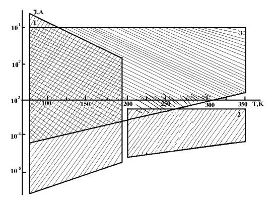
Fig. 1. Graph of the dependence of the maximum and minimum values of the amplitude of self-oscillations of the current on temperature,  $\rho = 5.104$  Ohm \* cm. 1-heating element (temperature-electrical instability); 2-PB (recombination waves): 3-IN (injection instabilities).
