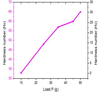
Fig.8. exposed load of Vickers hardness crystal of L-LMHCl - CA.
