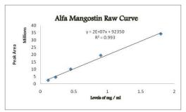
Figure 3. HPLC results for alpha mangosteen compounds
