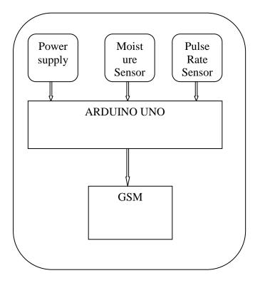
Figure 2: The Block diagram heart monitoring system
