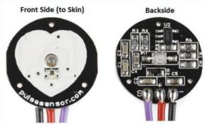
Fig. 4. Pulse rate sensor.
